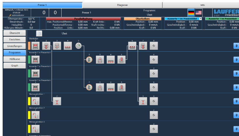
Figure 11: Freely programmable LaHMI sequence programming
